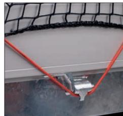
Extra, ingeniously-designed hinged bushes have been fitted to the H models. The useful hook makes it easy to attach the load net. A fixing point integrated in the side is available as an option.
