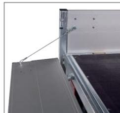
The H models have a U-profile at the rear. They also come prepared for the later addition of a storage compartment with drive-on ramps under the floor (with the exception of model H 260 x 150 cm).
