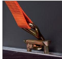
Each of the Azure models feature a binding bracket system integrated into the sides with a capacity of up to 1000 kg per piece as standard. This system is TÜV-certified.
