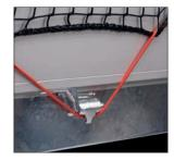
Extra, ingeniously-designed hinged bushes have been fitted to the HB and HM basic models. The useful hook makes it easy to attach the load net.
