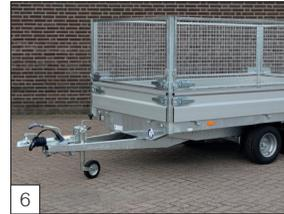
**Option:** removable and pendulating wire-mesh rack, provided with fasteners.
