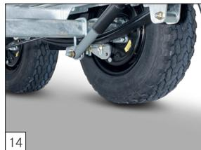
**Option:** the Azure H models in 3500 kg, from 335 x 180 cm, can be equipped with parabolic leaf spring axles including shock absorbers. Tyres 195/50 R13 and 185/70 R 13C are with black rims.
