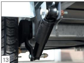
**Option:** shock absorbers mounted on axles.
