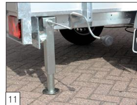
**Option:** adjustable, swivelling, telescoping prop stands and provided with removable crank.
