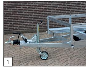
**Standard:** robust chassis, which is suitable for all single-axle versions up to and including 1800 kg Maximum Gross Weight.
