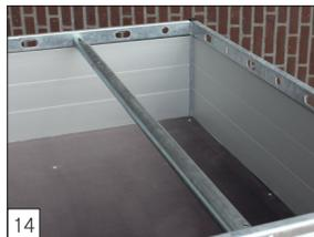
**Option:** load-restraint tubing mounted.
