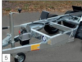
**Standard:** operated by a hand-pump and also a heavy jockey wheel is mounted.
