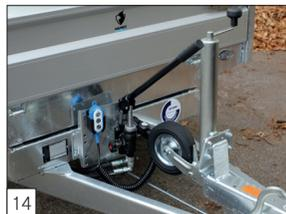
**Option:** an emergency hand pump (a removable control-box with spiral cable is as standard with the electric pump).
