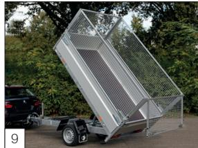
**Option:** removable wire-mesh rack with a height of 75 cm.
