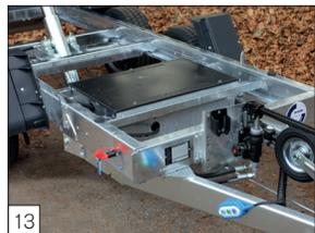
**Option:** electric control powered by a battery enclosed in a steel box.
