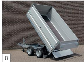
**Option:** aluminium dropsides with a height of 400 mm, pendulating.
