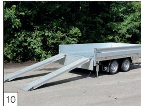
**Option:** a "DRIVE-ON"- kit mounted including 2 aluminium skids 2500 mm long with 2 heavy duty prop stands.
