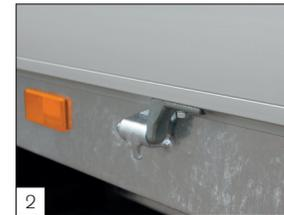
**Standard:** hook mounted around hinged points for easy mounting of accessories, including cargo net.
