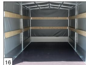
**Option:** a sloping roof is standard. HT models in 450 or 500 cm are as standard assembled with central posts on the sides.
