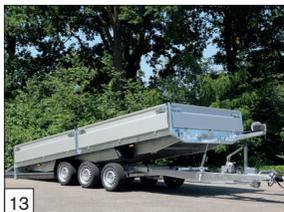
**Option:** models in 455 and 505 cm length are available as a 3 axle trailer and when with aluminium dropsides then the with removable centerposts.
